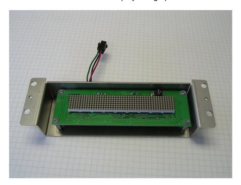
Remove paper and install red plastic filter, then reassemble stainless case.
