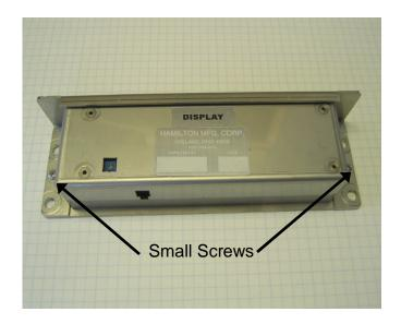
Remove screw and washer at each corner of display (4 places).
