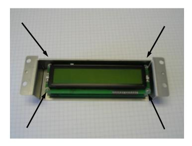
Carefully lift and separate two circuit boards.
