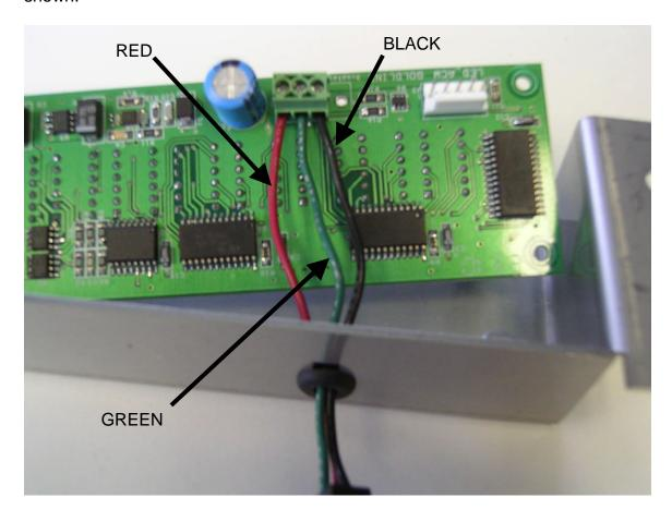
Turn board over and install on metal spacers as shown.
